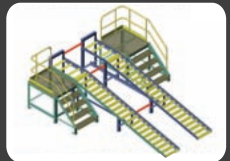
Light Vehicle Wash Down Ramp
